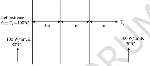
All slabs have thickness equal to 1 m and thermal conductivity of each slab is equal to 5  $Wm^{-1}$   $K^{-1}$ . The two extreme faces are exposed to fluid with heat transfer coefficient 100  $Wm^{-2}K^{-1}$  and bulk temperature 30°C as shown. The heat transfer in the slabs is assumed to be one dimensional and steady, and all properties are constant. If the left extreme face temperature  $T_1$  is measured to be 100°C, the right extreme faced temperature  $T_2$  is \_\_\_\_\_ °C.
