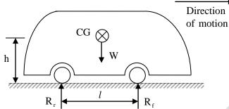
The distance between the front and rear wheels is  $\ell$ . The acceleration of the car is a, and acceleration due to gravity is g. The reactions on the front wheels (R<sub>f</sub>) and rear wheels (R<sub>r</sub>) are given by
