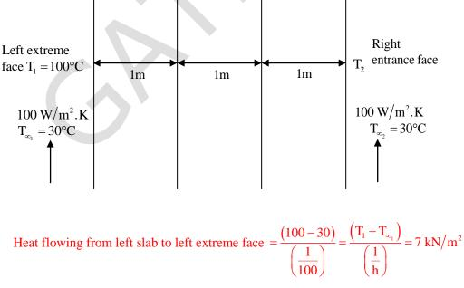
Heat generated in the central slab =  $10 \text{ kW/m}^3$
