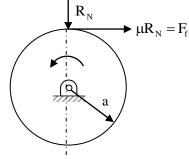
Given that Braking torque  $\tau_b = 250$  N.m
