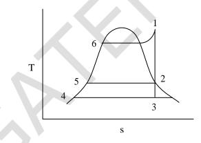
The mass flow rate of steam bled from the turbine as a percentage of the total mass flow rate at the inlet to the turbine at state 1 is \_\_\_\_\_.
