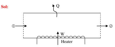
Inlet conditions  $P_1 = 100 \text{kPa}, T_1 = 27^{\circ}\text{C} = 300 \text{K}$   $V_1 = V_2 = 15 \text{ m}^3/\text{s}$  Q = -51 kWW = -101 kW
